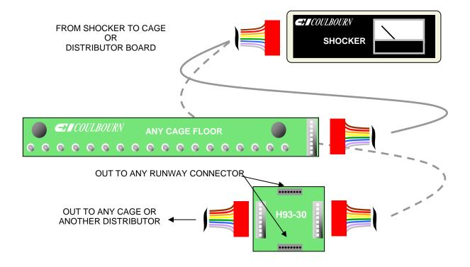
**NOTE:** RUNWAYS HAVE A CONNECTOR ON EACH SIDE TO ALLOW "DAISY-CHAIN" CONNECTIONS FROM RUNWAY TO RUNWAY USING ONLY H93-31-32 SHOCK CABLES
